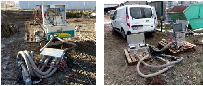
Figure 14: UBeG mobile TRT rig at the reference BHE in site A (left) and a smaller rig at the GEOCOND BHE in site B (right).
