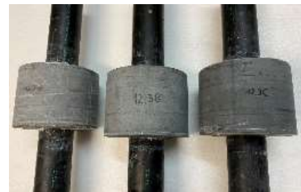
Figure 3: Tri-axial cells with samples of grout mix, seen at the end of a freezing phase (top) and samples of grout mix with central PE pipe, removed from the tri-axial cells after the end of the test cycles (bottom).
