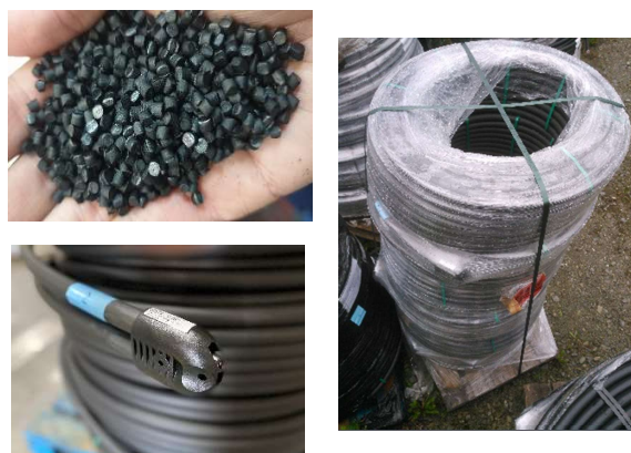
Figure 1: Pellets of Compound from Extruder at SILMA facilities (upper left), foot of a complete BHE manufactured by CAUDAL (lower left) and part of the coiled BHEs after arrival in Germany (right).
