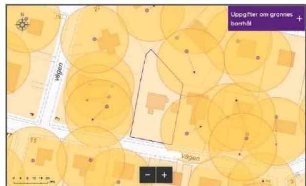
Figure 29: Example from the online application in Stockholm, a lot in a suburb without BHE and locations of existing BHE, from:
