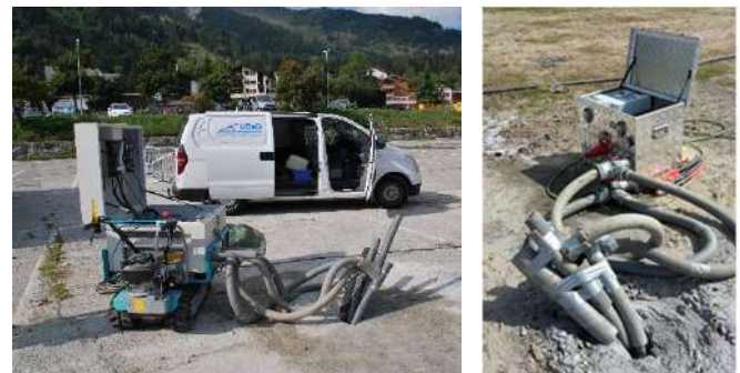
Figure 17: A German TRT rig, an insulated box moved on a crawler, on a site in Wallis, Switzerland in 2011 (left) and a small, portable TRT-device by the same company (right, photos Kahl).
