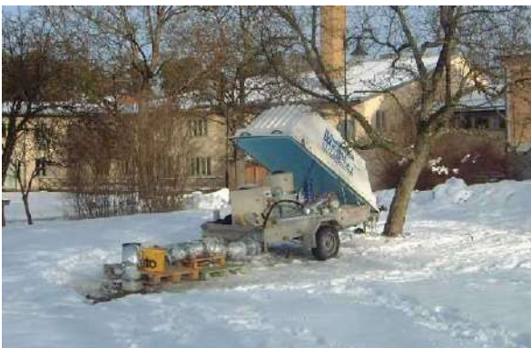
Figure 15: Swedish test rig, coupled to a borehole heat exchanger in the late 1990s.
