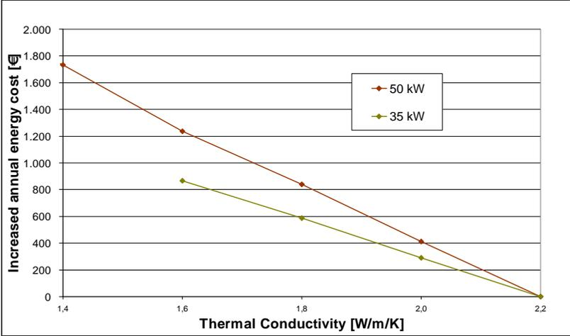
Figure 8: Effect of overestimation of thermal conductivity on the annual energy cost for sample 35 kW and 50 kW GSHP (see text)
