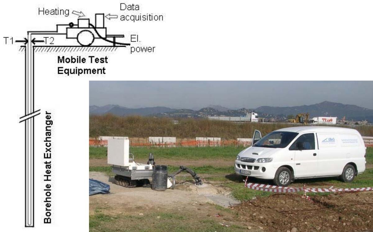
Figure 1: Schematic of TRT and photo of compact test rig (3<sup>rd</sup> generation UBeG GeRT), to be moved on a small crawler and transported in a van (example of rig from Germany transported to a test site in Northern Italy)
