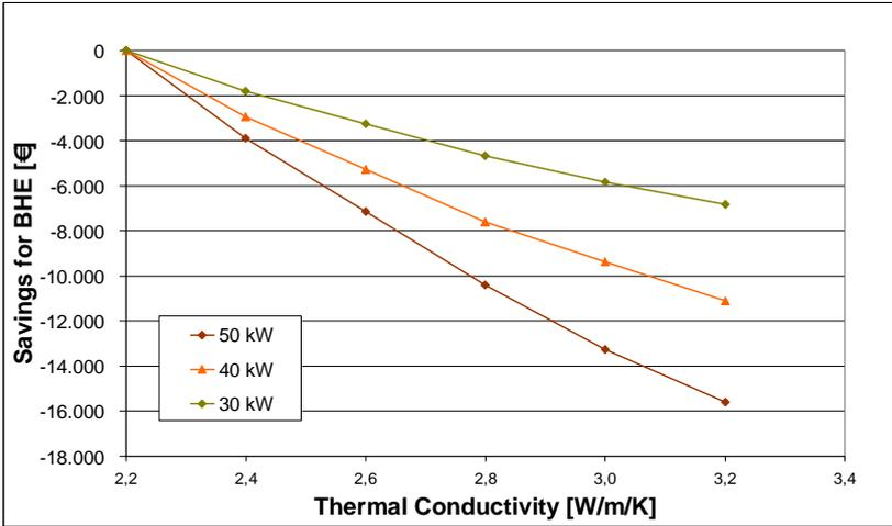
Figure 9: Effect of underestimation of thermal conductivity on cost for necessary BHE-field for sample 30-50 kW GSHP (see text)
