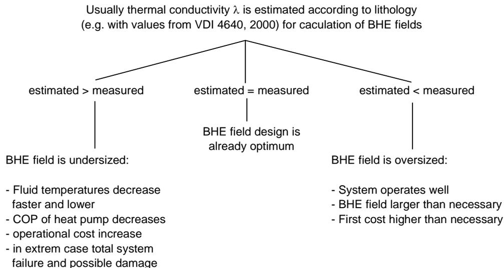
Figure 5: Possible consequences of error in estimated thermal conductivity values
