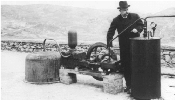
Fig. 2: First geothermal power production by Prince Ginori Conti at Larderello, Italy, in 1904, using a boiler heated from geothermal steam, a piston steam engine, and a dynamo (photo ENEL, Italy)
