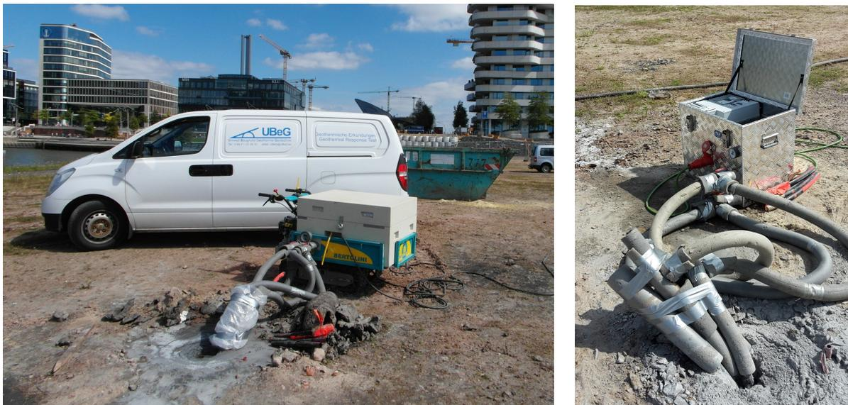
Figure 4: Typical TRT-setup at BHE on a site under development (left) and miniaturised, highly mobile TRT (right), both devised and built by UBeG (photos Kahl)
