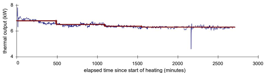
Figure 7: Thermal load curve for TRT from 2001 (TRT No. La3 in Table 4); a clear downward trend (decreasing thermal output) can be seen
