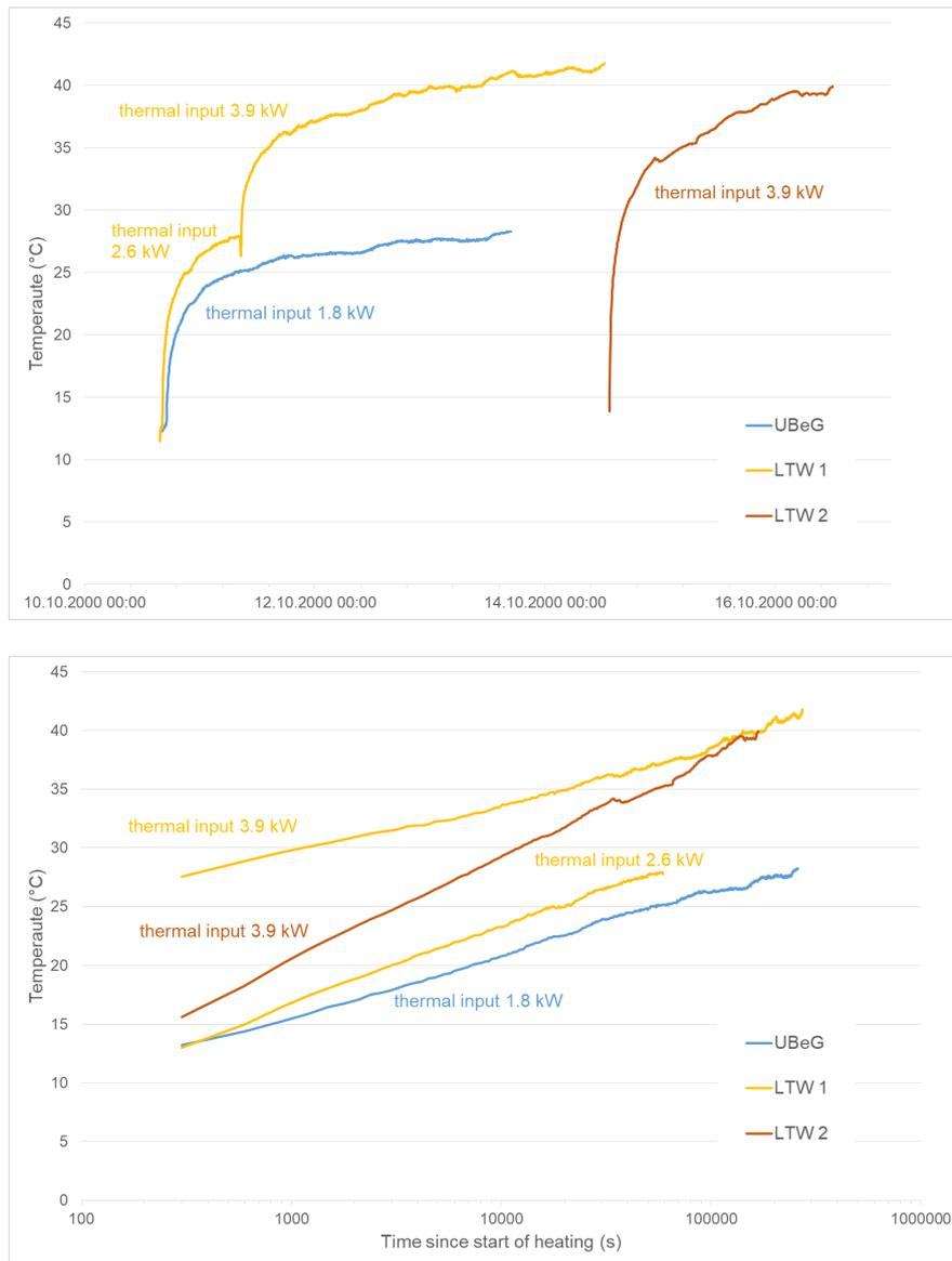
Figure 1: Development of the fluid temperature (mean of inlet and outlet) in three TRT performed in October 2000 in Mol, Belgium, by UBeG and Landtechnik Weihenstephan (LTW), on the real time axis (upper graph) and with logarithmic time (lower graph), plotted from the original data of IEA ECES Annex 13
