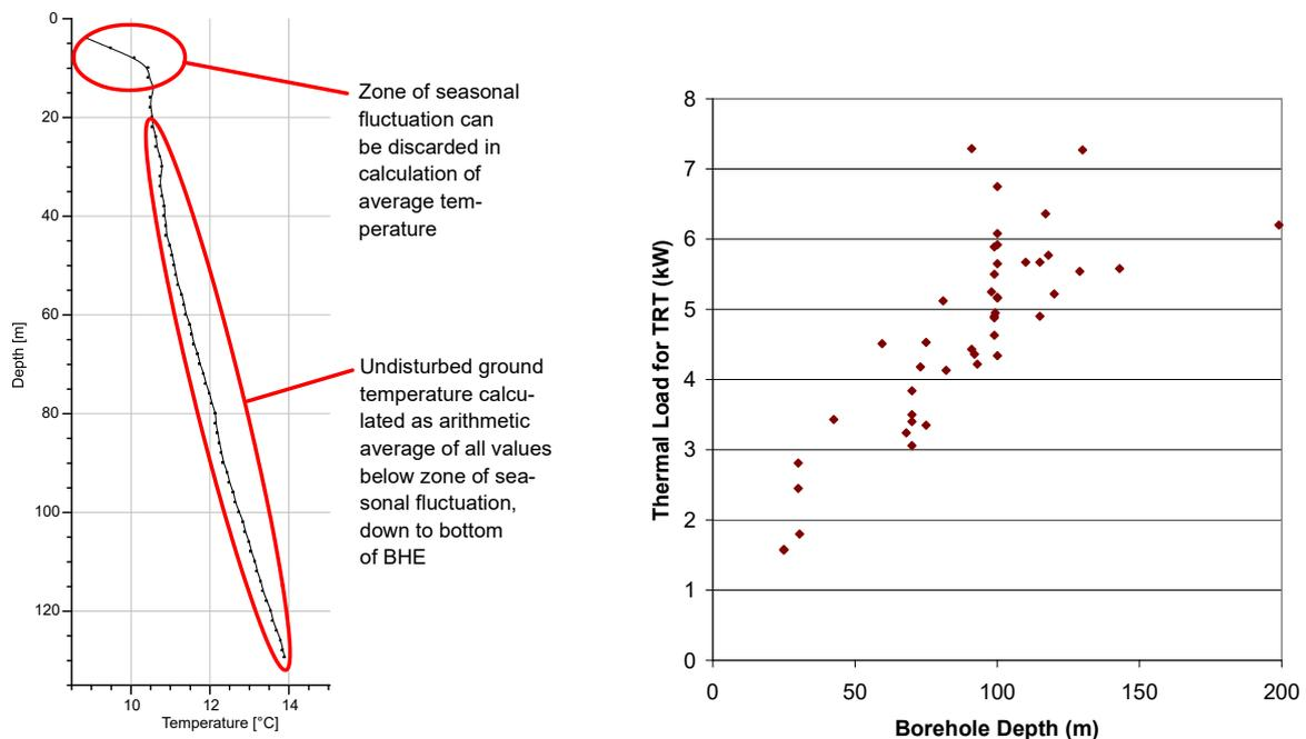
Figure 5: Example of temperature log in BHE to determine undisturbed ground temperature (left, taken towards the end of winter) and thermal load for TRT versus borehole depth for a number of tests (right)
