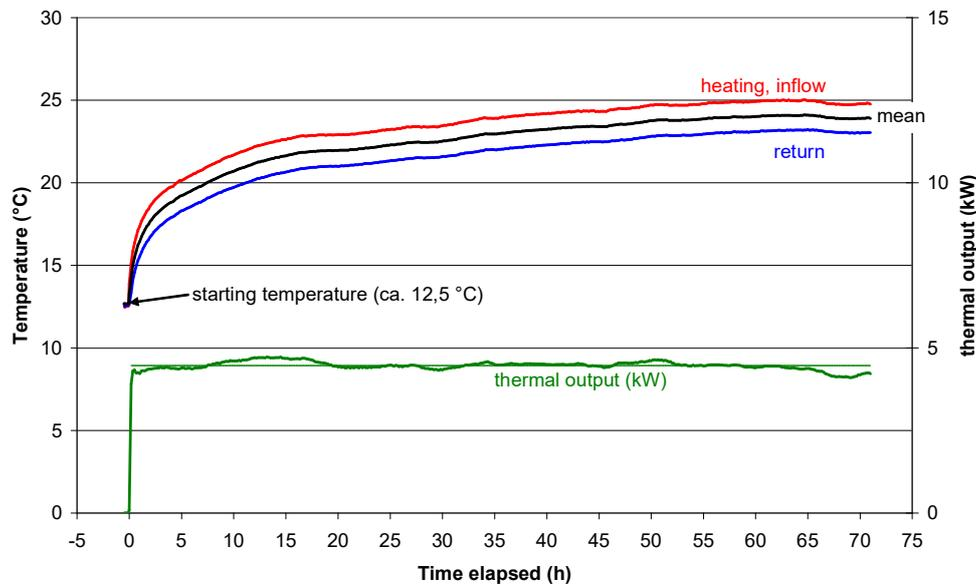
Figure 6: Example of temperature and load curve for TRT, from real data over >70 hours; small fluctuations in thermal load can be seen, but no upward or downward trend
