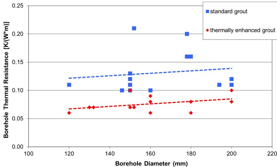
Figure 8: Borehole Thermal Resistance from 31 TRTs made in Germany in 1999-2004, BHE grouted with standard or thermally enhanced grout (after Sanner et al, 2005)
