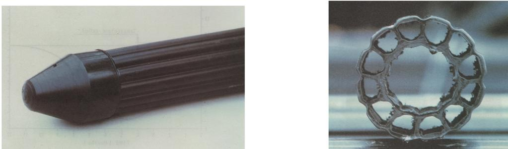
Figure 3: Coaxial BHE by SHF in Switzerland, made of PE with multi-chamber outer channel for turbulent flow and increased heat exchange (photos from Hess, 1987)
