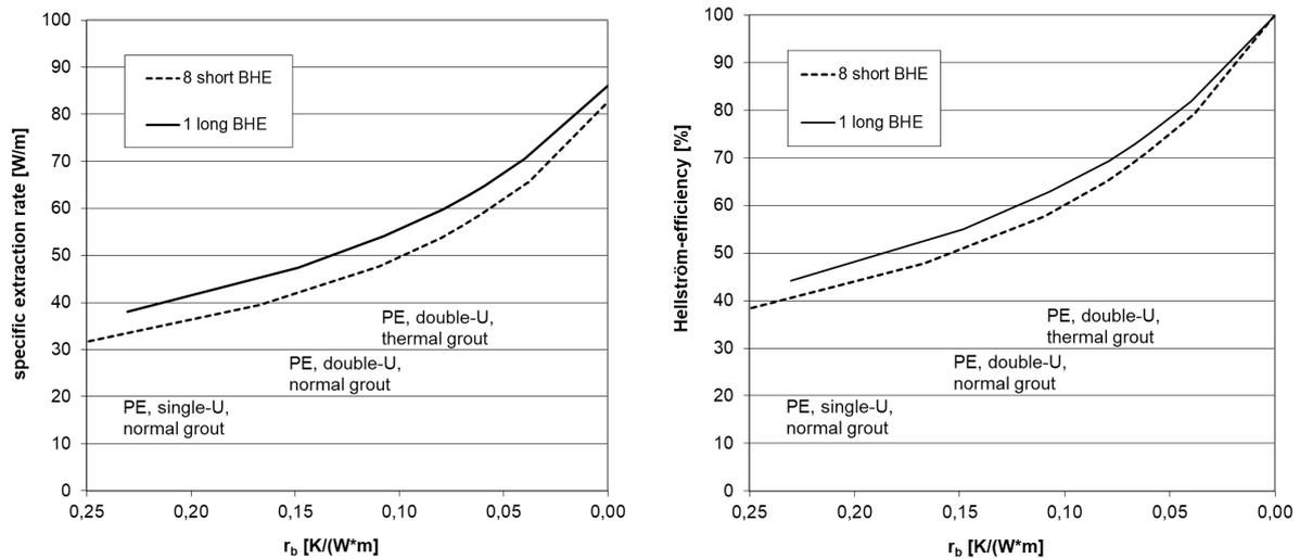
Figure 9: Achievable specific heat rate in a sample GSHP (left) and concept of Hellström-efficiency  $\eta_H$  (right, see text); plotted against  $r_b$ -value, areas of typical BHE-types indicated
