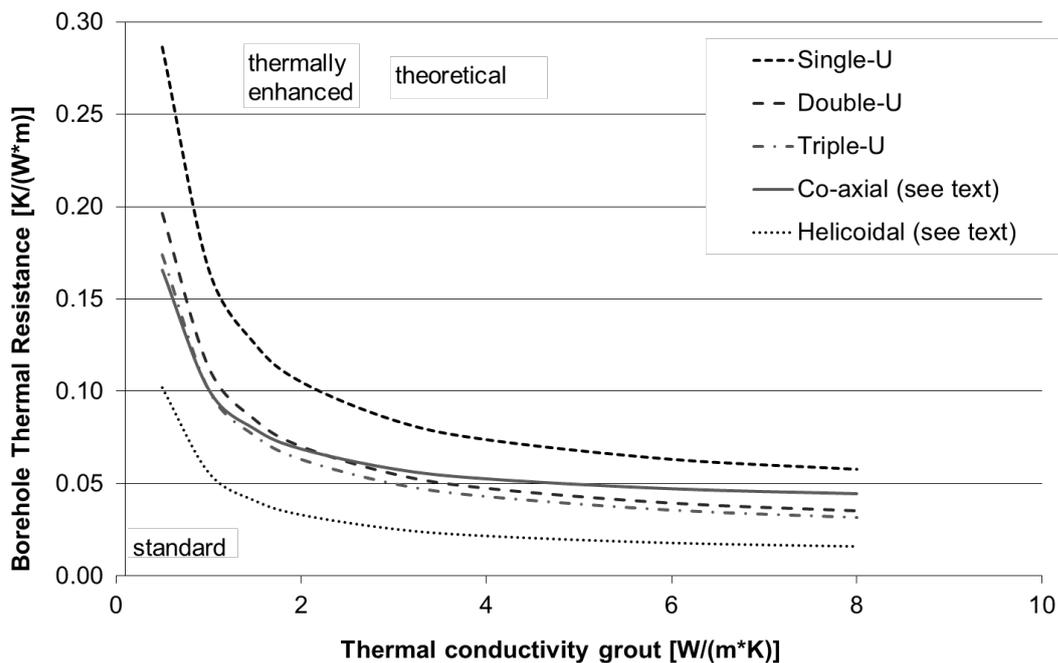
Figure 7: Borehole Thermal Resistance for different configurations versus thermal conductivity of grout (backfilling); helicoidal by approximation only
