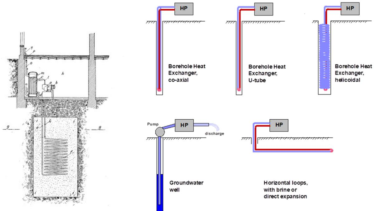
Figure 1: Left – Ground Source Heat Pump in Swiss Patent 59350 of 1912 (inventor H. Zoelly); Right – Ground-coupling methods listed by Kemler (1947), re-drawn and harmonised as in Sanner (2005)
