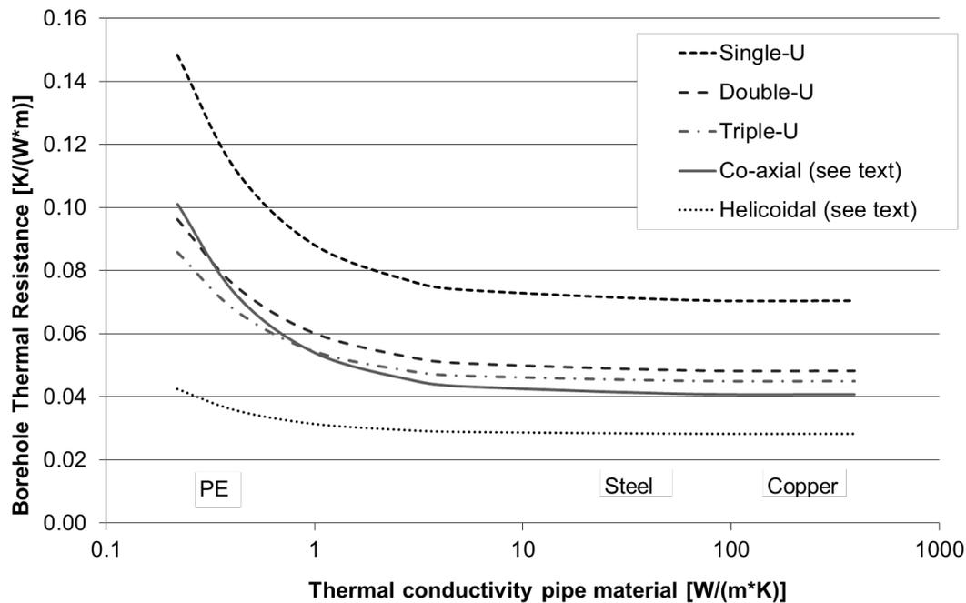
Figure 6: Borehole Thermal Resistance  $r_b$  for different configurations versus thermal conductivity of pipe material, see text for details; helicoidal by approximation only
