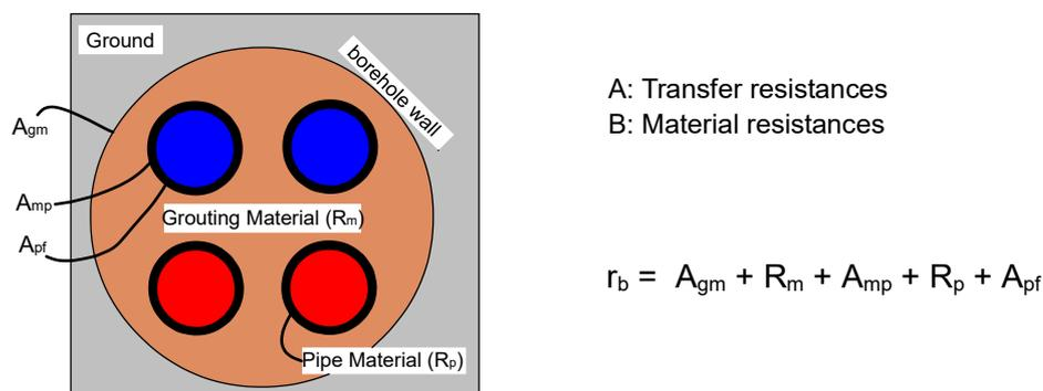
Figure 5: Components of borehole thermal resistance  $r_b$  for a double-U-BHE
