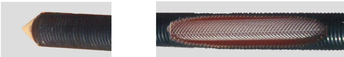
Figure 2: Coaxial BHE as tested in Schwalbach GSHP research station (Sanner, 1986), consisting of corrugated metal outer tube (usually stainless steel, but copper in this cut-out sample for exhibitions), protected against corrosion by a PE-coating
