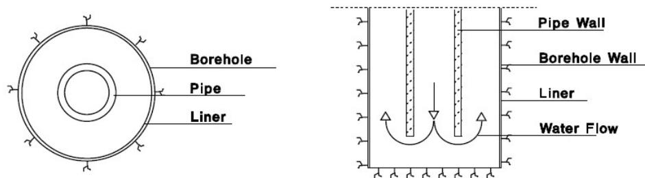
Figure 4: Coaxial BHE in open borehole (with or without liner, depending on rock quality) as used in Luleå BTES, constructed 1982/83 (graph from Nordell, 1994)
