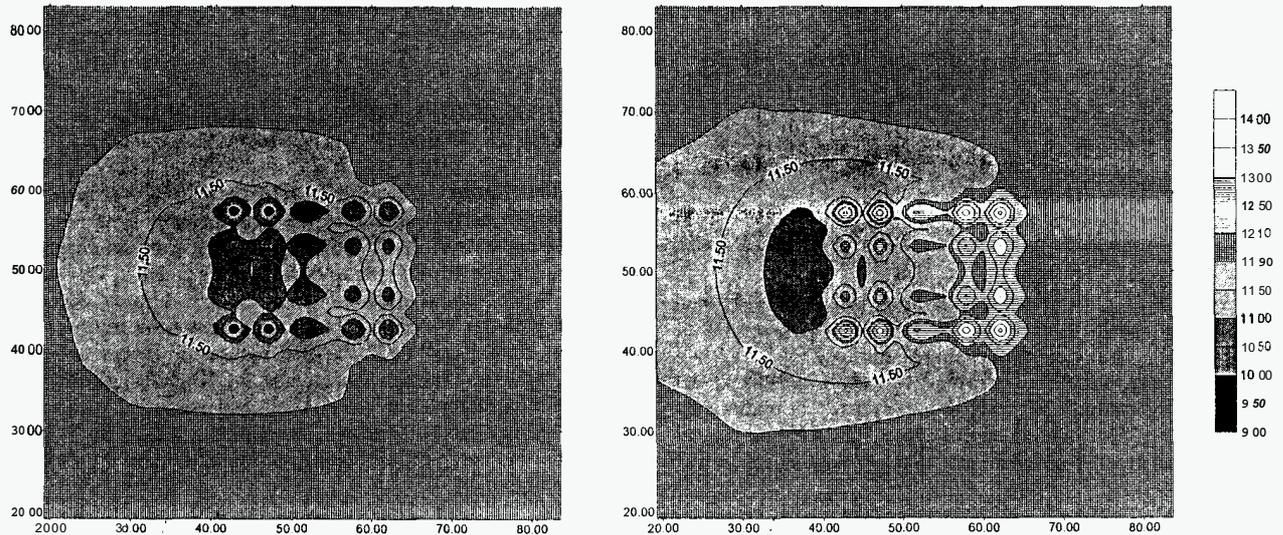
Figure 15: Temperature distribution around one cluster with 20 vertical earth heat exchangers, project "Reichstag" building, Berlin; left January 1st, right September 1st in the second year of operation. The axes are given in meter, the isotherms in centigrade.
