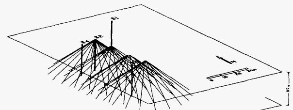
Figure 11: layout of "Technorama" Düsseldorf earth heat exchangers.
