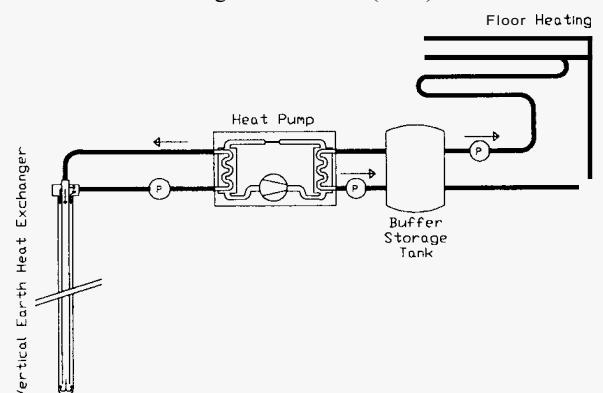
Figure 1: Schematic of "conventional" GSHP in Mid Europe
