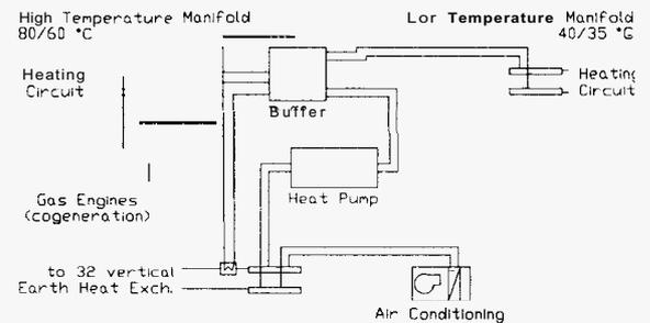
Figure 8: Schematic of GSHP-plant Frankfurt-Hochst
