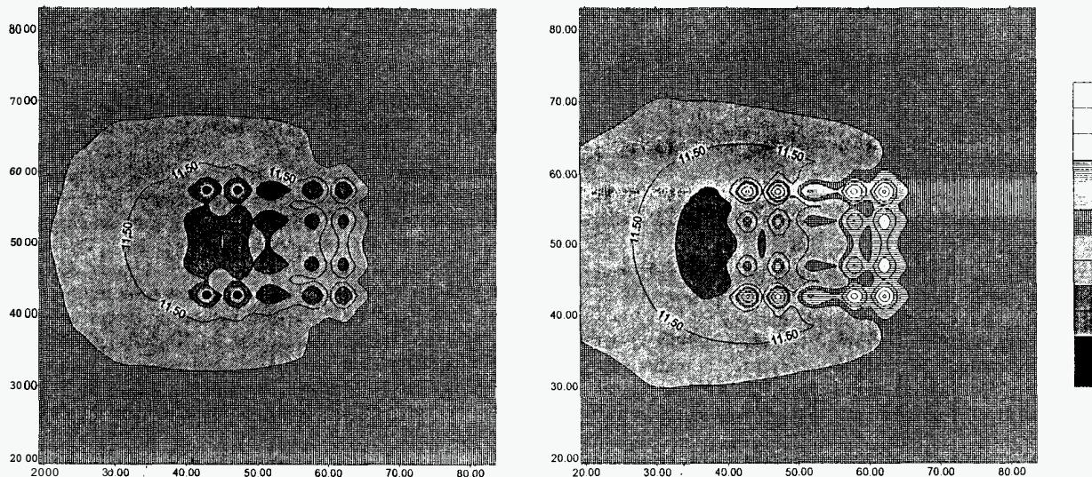
Figure 15: Temperature distribution around one cluster with 20 vertical earth heat exchangers, project "Keichstag" building, Berlin; left January 1st, right September 1st in the second year of operation. The axes are given in meter, the isotherms in centigrade.
