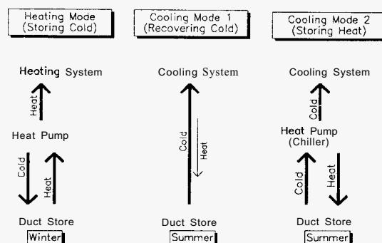
Fig. 9: Operation principles of GSHP-plants with cold storage
