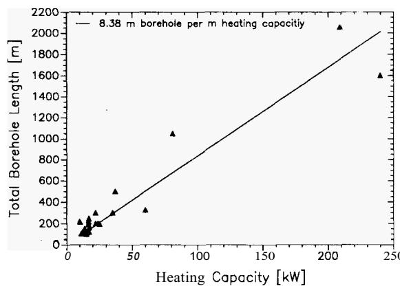
Figure 3: Borehole length versus Heat Pump Heating Capacity for 20 European GSHP-plants.
