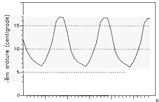
Figure 14: Monthly average brine temperatures for the first three years of operation, project "Reichstag" building, Berlin; storage with 160 vertical earth heat exchangers.
