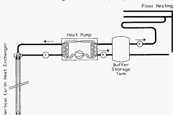
Figure 1: Schematic of "conventional" GSHP in Mid Europe
