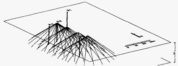
Figure 11: layout of "Technorama" Diisseldorf earth heat exchangers.
