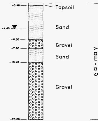
Figure 10: Geological profile at the GSHP-site Dusseldorf
