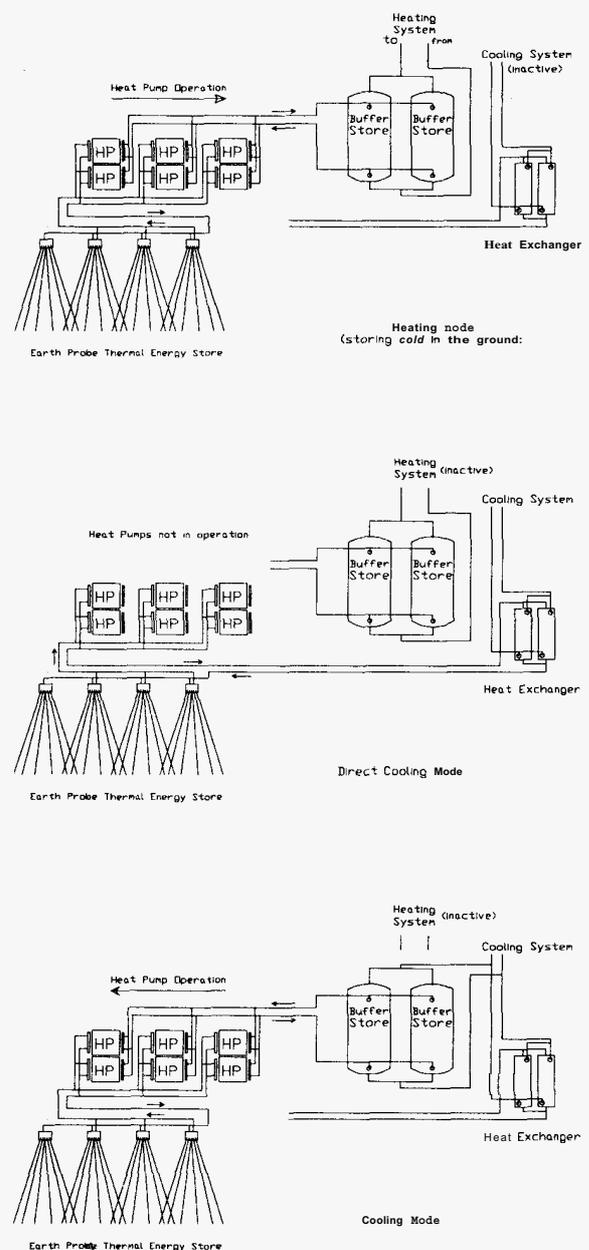
Figure 12: Schematic of "Technorama" Diisseldorf GSHP cold storage plant in 3 operation modes.
