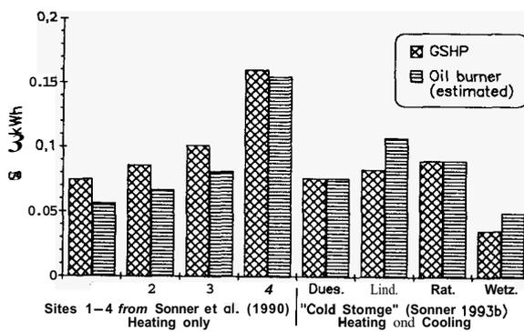
Figure 13: Cost of heating/cooling energy per kWh, incl. capital cost, in comparison to conventional design
