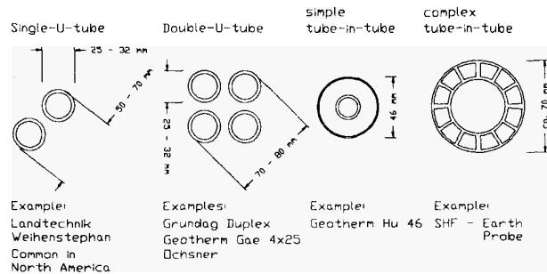
Figure 2: Cross-sections of typical vertical earth heat exchangers
