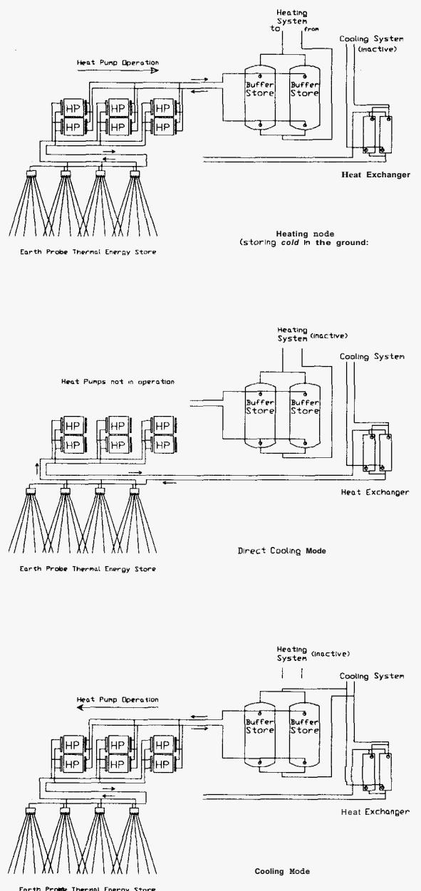
Figure 12: Schematic of "Technorama" Düsseldorf GSHP cold storage plant in 3 operation modes.
