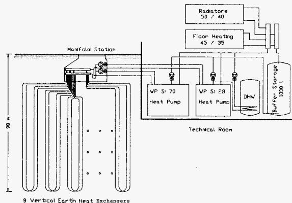
Figure 6: Schematic of a sub-system of GSHP plant Kochel a.S.
