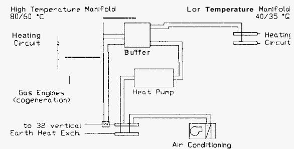
Figure 8: Schematic of GSHP-plant Frankfurt-Hiichst
