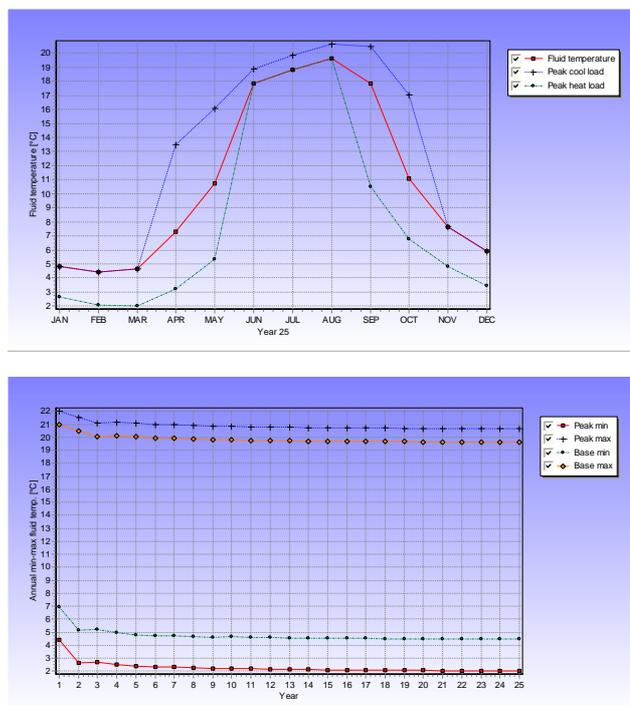
Figure 4: Temperature development in the BHE in the 25<sup>th</sup> year of operation, and minimum and maximum temperatures over the simulation period of 25 years, calculated with EED.
