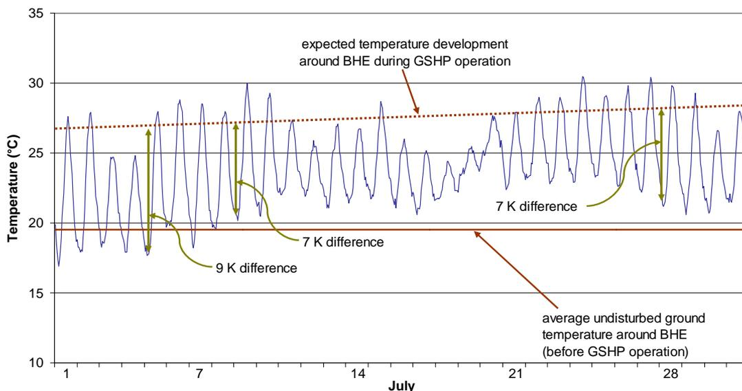
Figure 2: Hourly dry air temperature in July (data for Cadiz, from Spanish Meteorological Service) and ground temperatures in undisturbed situation and during GSHP operation
