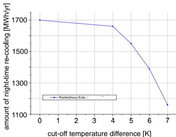
Fig 10: Amount of annual re-cooling from night-time operation against the cut-off temperature difference
