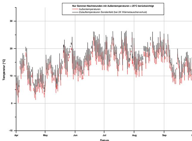
**Fig 7: Average night temperatures (red) and possible recharge temperatures (black) from April to September**
