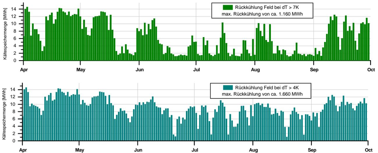
Fig 9: Amount of re-cooling for different temperature differences for cut-off; example for 7 K (above) and 4 K (below).
