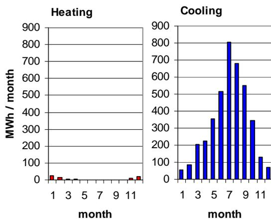
**Figure 1: Monthly heating and cooling loads as to building design for Jerez retail outlet**
