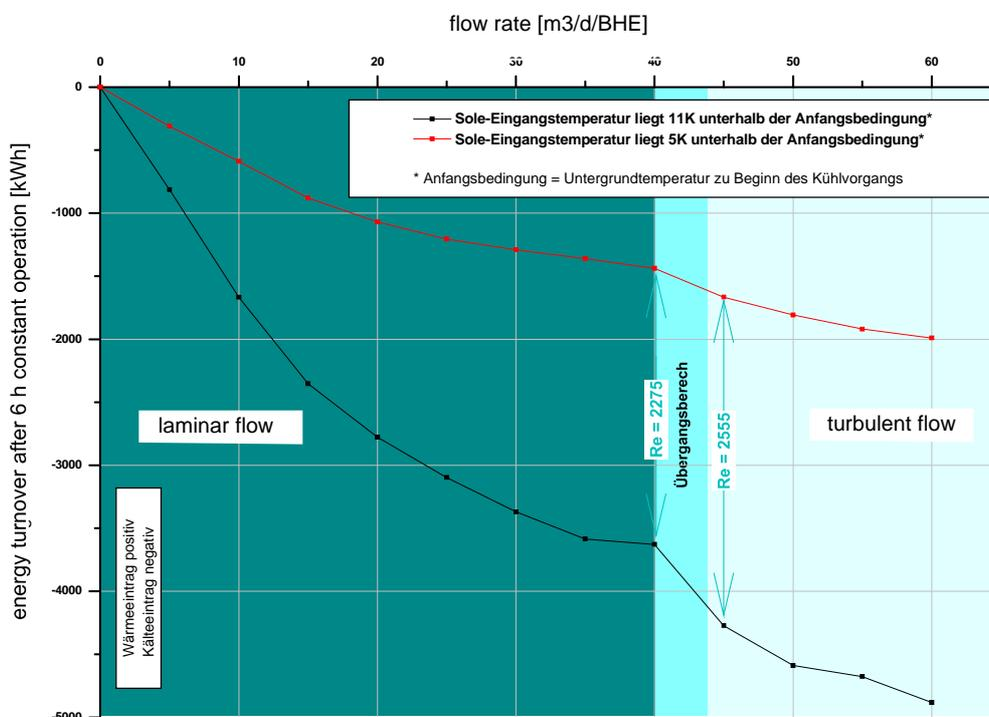
**Fig 8: Flow-rate and re-cooling of the underground**
