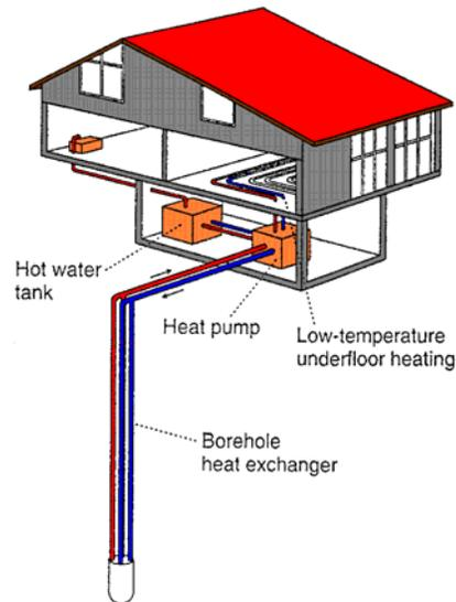
**Fig. 3: Typical application of a BHE / heat pump system in a Central European home, typical BHE length ≥100 m**
