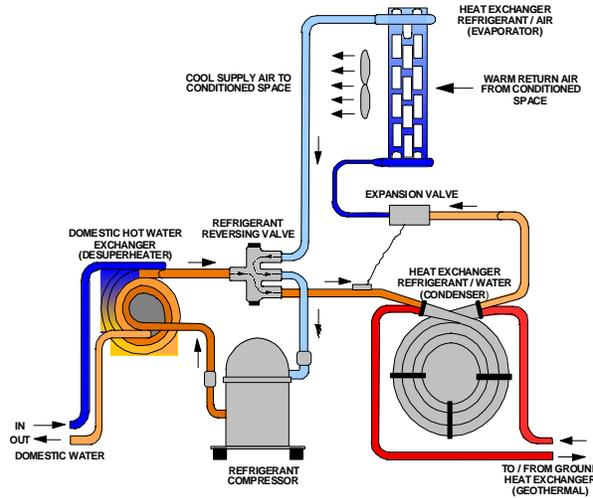
**Figure 1a. Water to air GHP in the cooling cycle (source: Oklahoma State University)**
