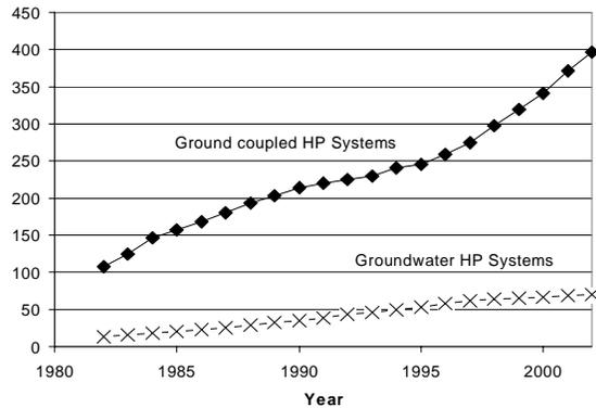
**Figure 7. Development of installed capacities (MWt) of BHE-coupled (top) and groundwater-based (bottom) geothermal heat pumps in Switzerland during the years 1980 - 2001 (from Kohl et al., 2002).**
