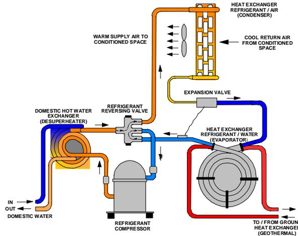
**Figure 1b. Water-to-air GHP in the heating cycle (source: Oklahoma State University)**
